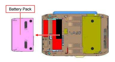
In the state of 1), remove the Battery Pack in the direction of the arrow.
