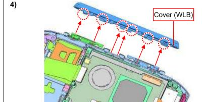
Disengage the detent (six places) and remove the Cover. *UX Series*  1.MS-1-D.11 Confidential
