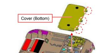
While disengaging the detent (three places), remove the Cover.
