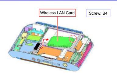
Remove the one screw and then the Wireless LAN Card.
