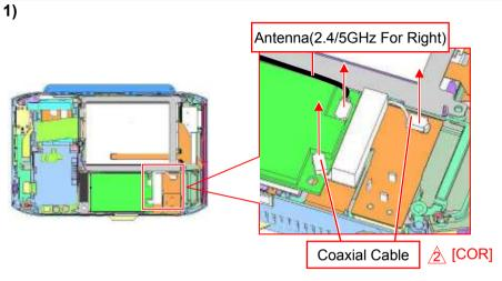
Disconnect the Antenna (one place) and the terminal of the Coaxial Cable (two places) **vertically**.
