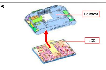
While disengaging the detent (four places), remove the Palmrest.
