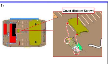
While disengaging the detent (two places), remove the Cover.
