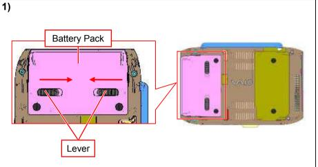
Turn over the main unit, and slide the lever in the direction of the arrow to release the lock.
