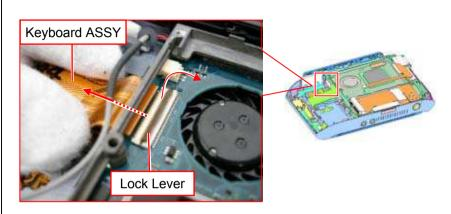
Raise the lock lever to release the lock and remove the Keyboard ASSY.
