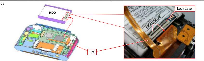
2. While disconnecting the FPC, remove the HDD.
