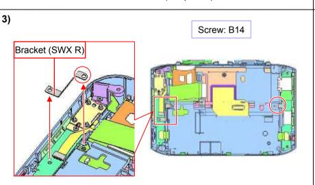
Remove the two screws and the Bracket.
