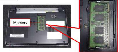
The Memory on side B of the Mother Board can be removed.
