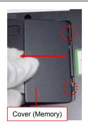
Hook a finger on the A portion, raise the Cover, and remove it in the direction of the arrow.
