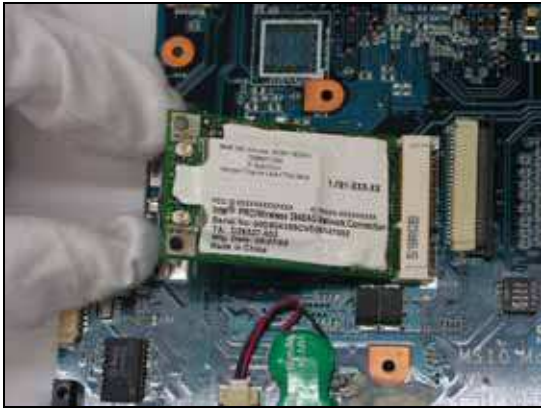
Step 36. Turn around the WHU and unlock the socket as shown.
