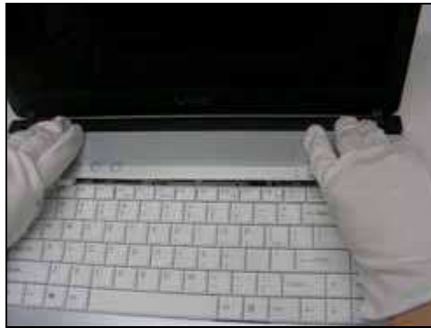
Step 12. Remove the K/B cover and set aside.
