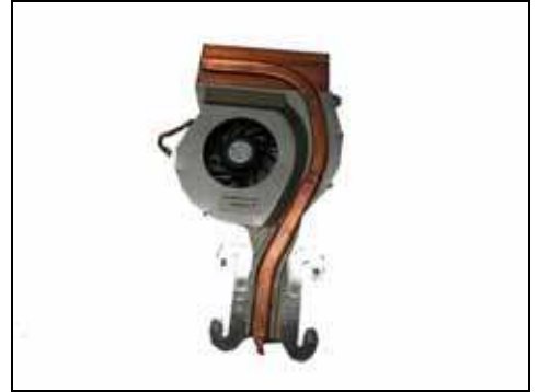
Step 32. Gently remove the ASSY Thermal CPU and set aside.
