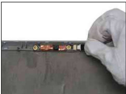
Step 23. Gently pull out the cable.
