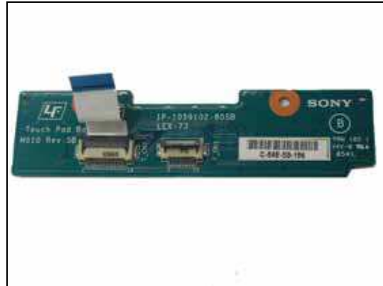
Step 39. Remove the PWBA touchpad.
