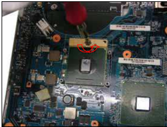
Step 33. Unlock the CPU socket in the direction of arrow then remove the CPU.
