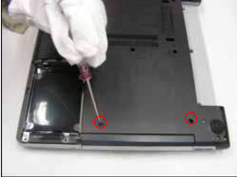
Step 9. Using a screwdriver, remove the marked screw.
