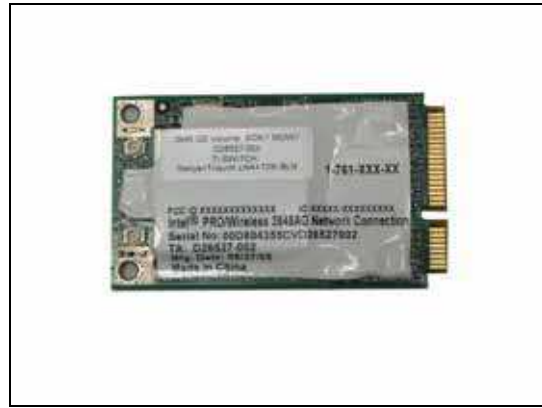
Step 37. Remove the WLAN card and set aside.
