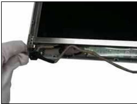
Step 22. Gently remove the Hinge and LCD panel.
