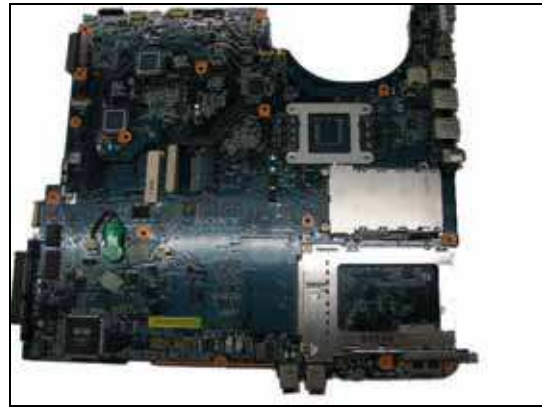
Step 39. Remove the M/B and set aside.
