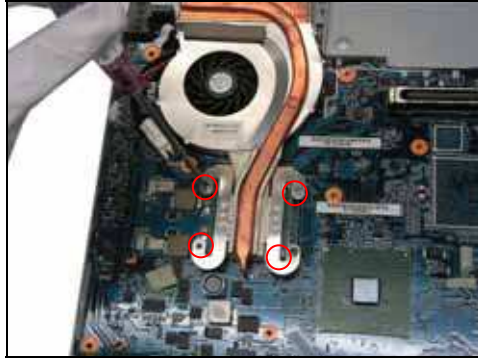
Step 31. Using a screwdriver, remove the marked screw.
