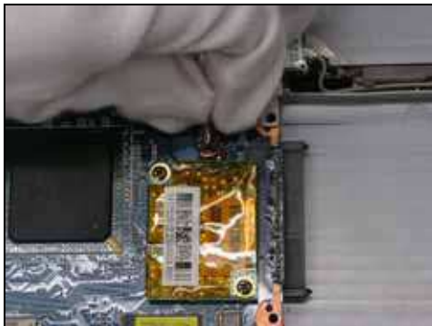
Step 34. Gently remove the Modem cable.
