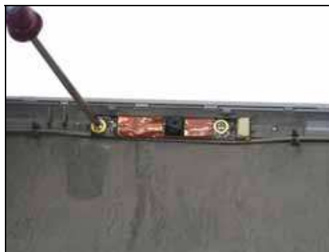
Step 24. Using a screwdriver, remove the marked screw.
