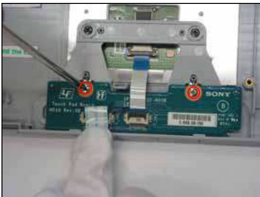
Step 40. Remove the marked screw and cable.
