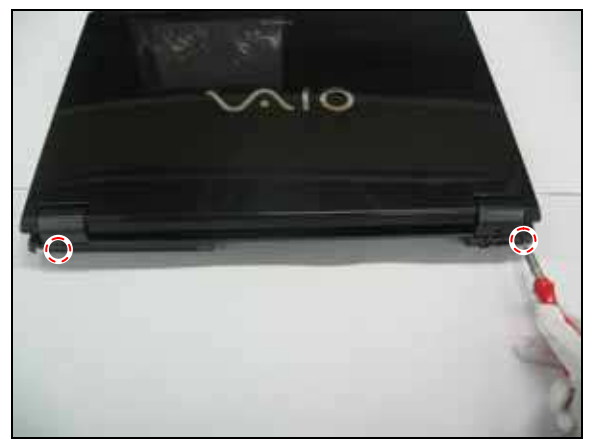
Step 17.Close the LCD, turn the reverse side of the notebook upward and Use a screwdriver to remove the marked screw. Then remove the two screws of the Hinge Cover.
