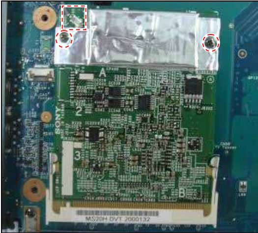
Step 35. Remove the marked two cables. Use a screwdriver to remove the marked two screws.
