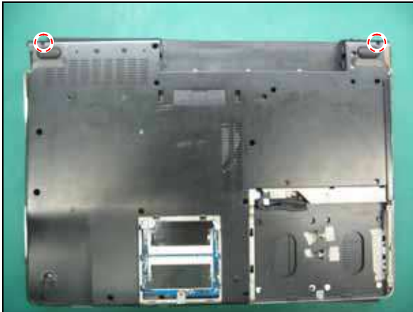
Step 17.Close the LCD, turn the reverse side of the notebook upward and Use a screwdriver to remove the marked screw. Then remove the two screws of the Hinge Cover.
