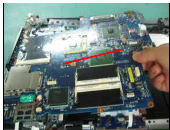
Step 59. Lift the Mother Board up from the right side and remove to the right.
