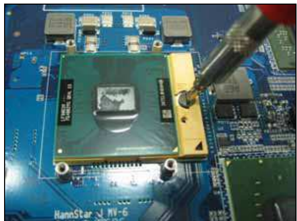
Step 49. Use a screwdriver to rotate the screw 180 degree. Gently remove the CPU.
