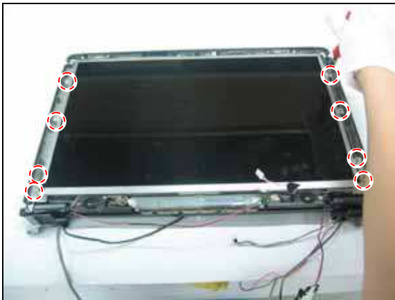
Step 25. Use a screwdriver to remove the marked eight screws.
