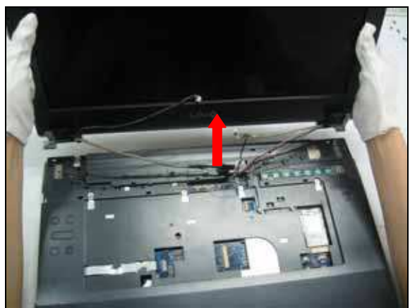
Step 18. Gently pull out the LCD.
