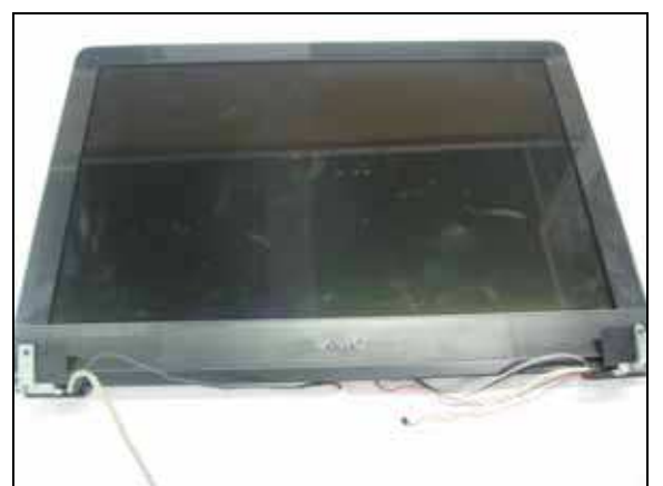
Step 17.Close the LCD, turn the reverse side of the notebook upward and Use a screwdriver to remove the marked screw. Then remove the two screws of the Hinge Cover.
