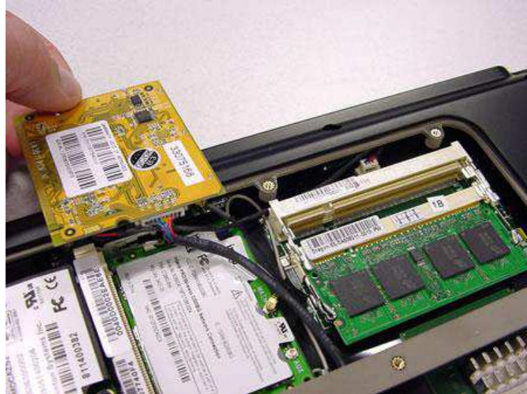
Fig. 5 Removing the Mini-PCI wireless card.
