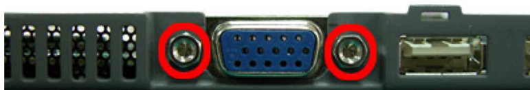
Fig. 34 Disconnecting the VGA connector
