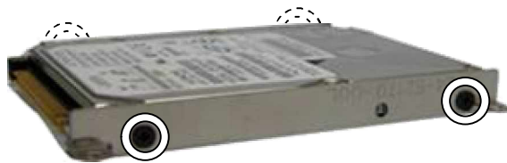
Fig. 4 Unscrewing the hard disk drive bracket screws
