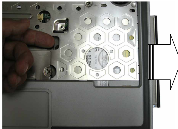
Fig. 11 Pushing Optical Drive module out from base unit
