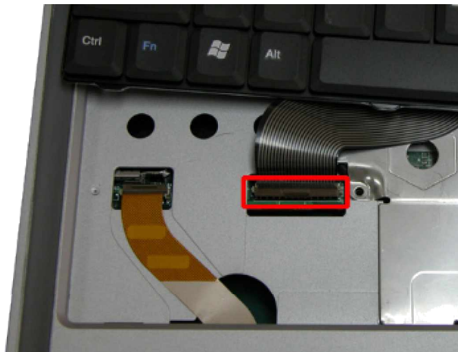
Fig. 9 Removing the keyboard FPC cable
