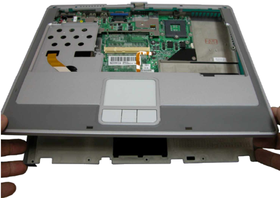
Fig. 29 Removing the top cover
