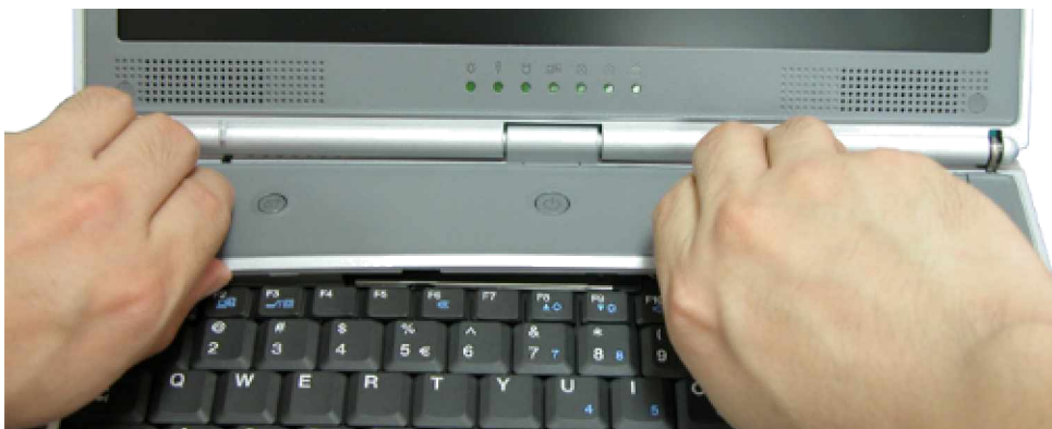
Fig. 7 Removing the Keyboard Cover
