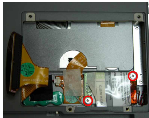
Fig. 5 Removing the screws on the MCD modem
