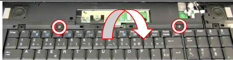
Fig. 12 Location of keyboard screws.
