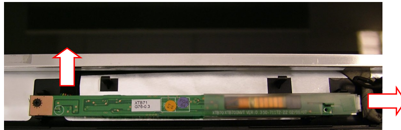
Fig. 43 Disconnecting cables from inverter board.
