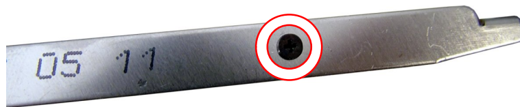
Fig. 45 Location of screw securing brackets.
