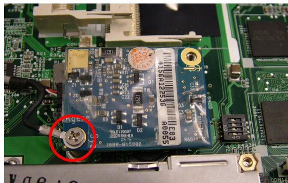
Fig. 18 Removing the modem screw.
