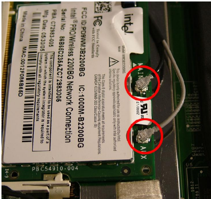
Fig. 11 The 2 antenna connectors: MAIN and AUX.
