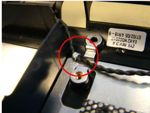
Fig. 23 Metal clip securing the speaker cable.
