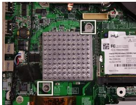
Fig. 26 Location chipset heat sink screws.
