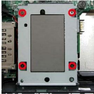
Fig. 29 Screw location on the HDD holder.
