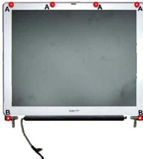
Fig. 16 Location of rubber covers and screws.
