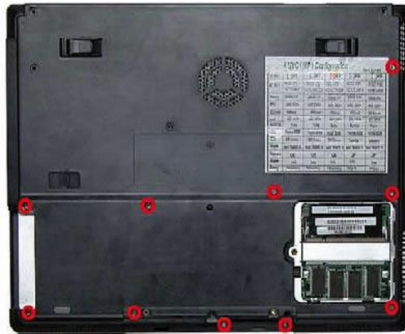
Fig. 22 Location bottom cover screws.
