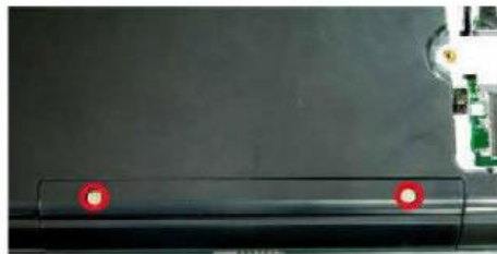
Fig. 4 Removing the hard disk drive cover.
