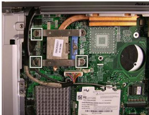
Fig. 20 Location remaining CPU heat sink screws.
