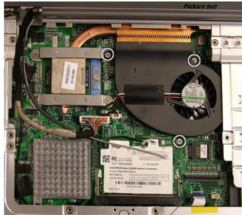
Fig. 19 Location CPU fan screws.
