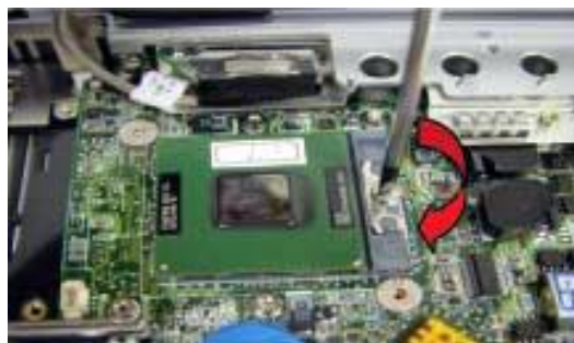
Fig. 21 Removing the CPU.
