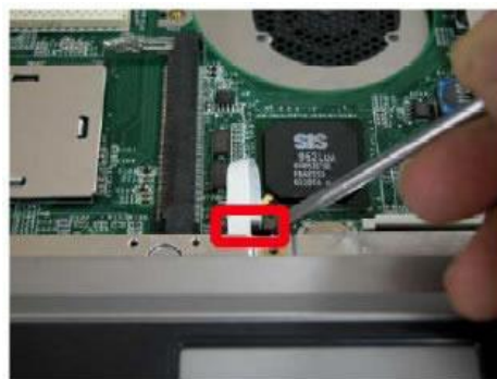
Fig. 24 Disconnecting the touchpad cable.
