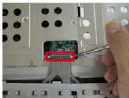
Fig. 8 Disconnecting the keyboard flat cable.
