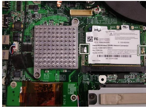
Fig. 27 Releasing the WLAN side locks.
