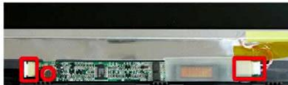
Fig. 17 Removing the inverter board.
