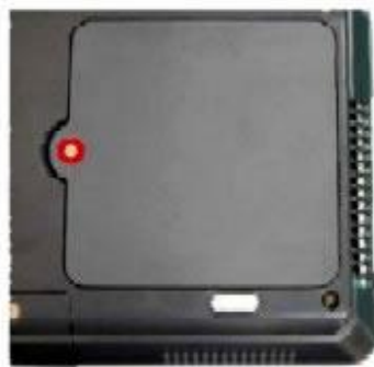
Fig. 2 Memory compartment cover screw location.
