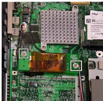
Fig. 28 Location modem card screws.
