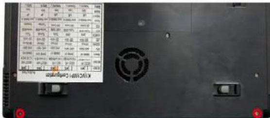
Fig. 13 Removing the LCD module screws (bottom).
