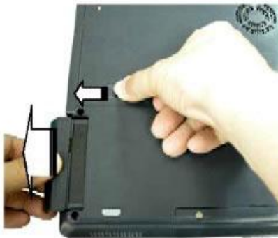
Fig. 1 Releasing the battery.
