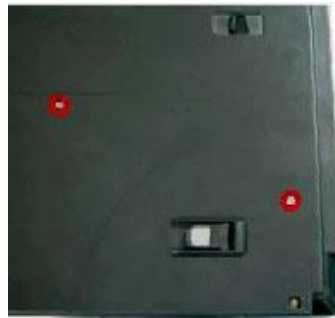
Fig. 10 Releasing the optical disk drive.
