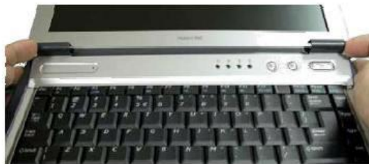
Fig. 7 Lifting the keyboard.
