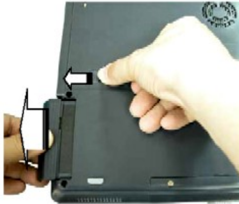
Fig. 1 Releasing the battery
