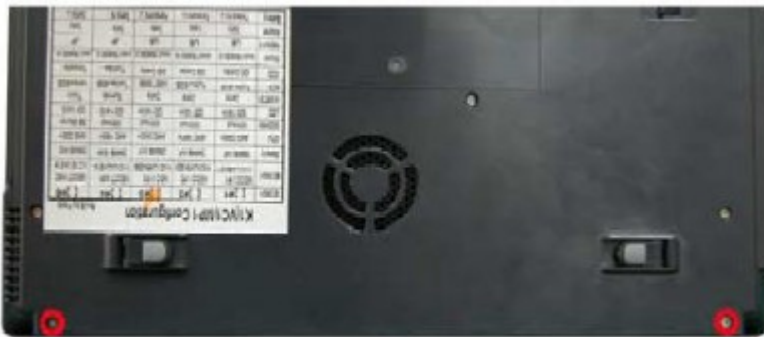
Fig. 12 Bottom screws retaining the LCD Module
