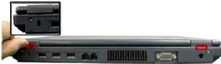
Fig. 6 Releasing the keyboard cover
