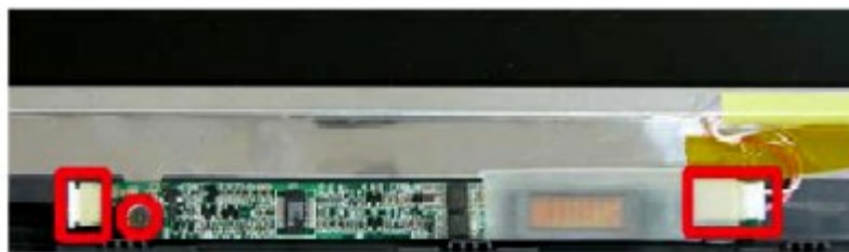
Fig. 16 Removing the Inverter Board
