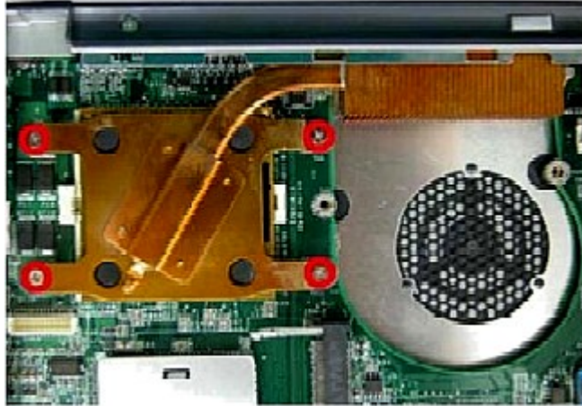
Fig. 20 Removing the CPU heat sink screws
