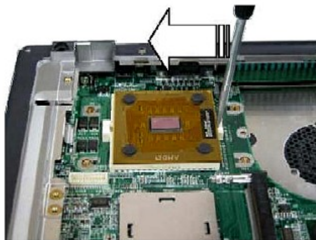
Fig. 21 Unlocking the CPU
