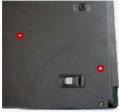
Fig. 9 Releasing the optical disk drive
