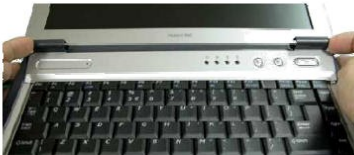
Fig. 7 Lifting up the keyboard cover
