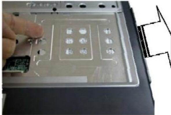
Fig. 10 Pushing the optical drive out
