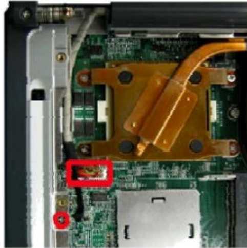
Fig. 14 Removing the screws retaining the LCD Cable Connector
