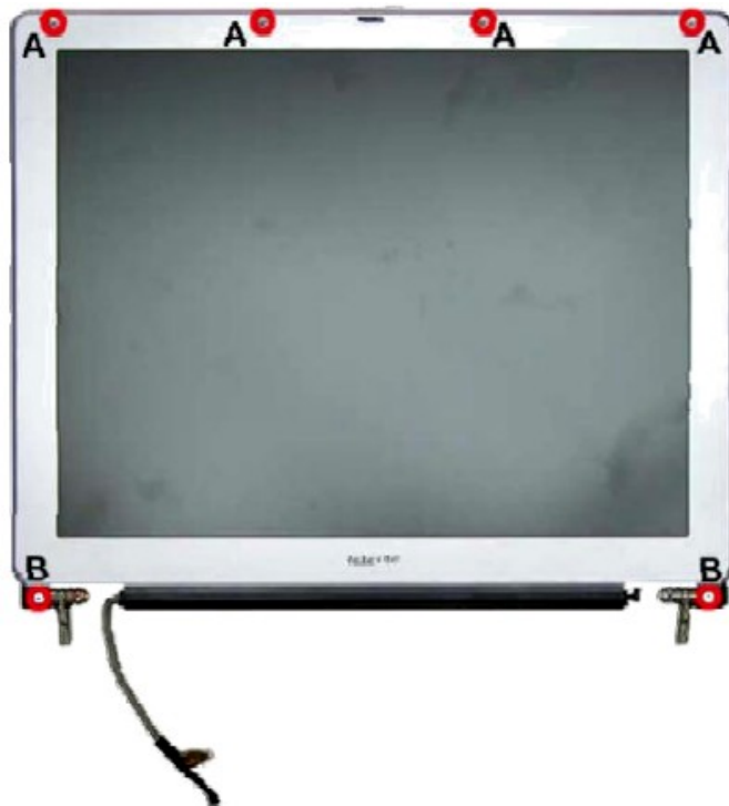
Fig. 15 Removing the rubber covers & screws on the LCD Module
