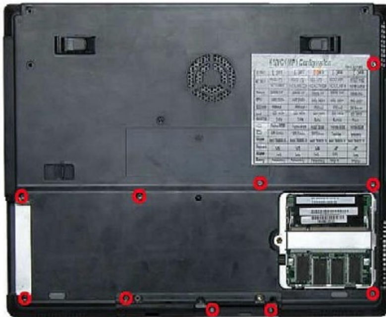
Fig. 22 Bottom cover screws
