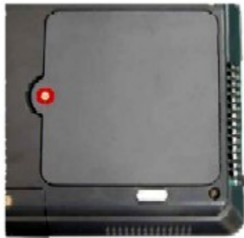
Fig. 2 Removing the screw retaining the memory cover
