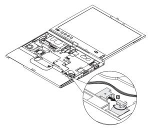
Gently lift upper case up, as shown in step [4] and [5], to remove upper case.
