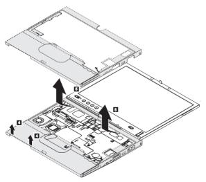
When installing: Follow the steps below to make sure that the upper case is installed firmly.
