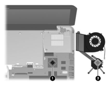
Reverse this procedure to install the video fan/heat sink assembly.
