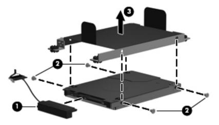
Reverse this procedure to reassemble and install the hard drive.
