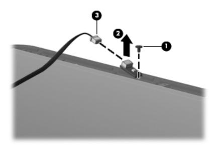
d. Remove the ambient light sensor module. The ambient light sensor module and cable are available using spare part number 576815-001.
