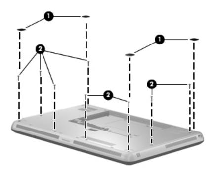
2. Remove the two Phillips PM2.0×5.0 screws **1** and the four Phillips PM2.0×2.0 screws **2** that secure the top cover to the base enclosure.
