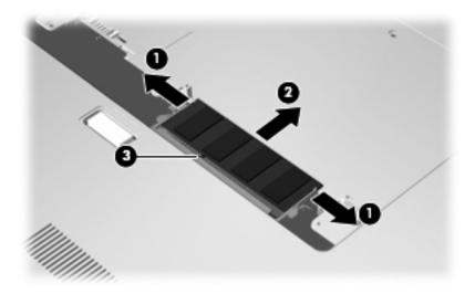
Reverse this procedure to install the expansion memory module.
