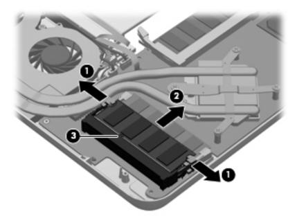
Reverse this procedure to install the primary memory module.
