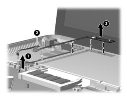
3. Remove the power button board and cable.
