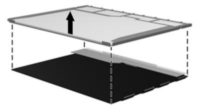
24. Recycle the LCD panel and backlight.
