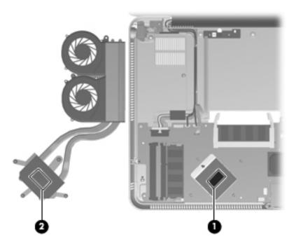
Reverse this procedure to install the processor fan/heat sink assembly.
