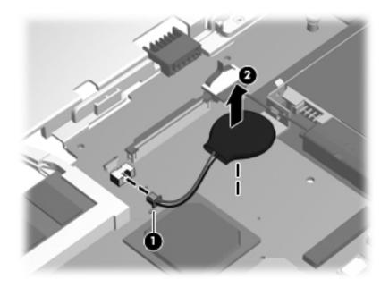
3. Remove the RTC battery.
