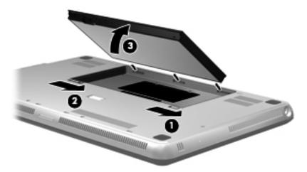
Install the battery by aligning the tabs on the battery with the notches on the outer edge of the battery bay, and then lowering the battery into the battery bay until it is seated. Slide the battery lock to lock the battery into place.
