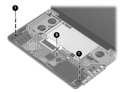
Where used: 4 screws that secure the system board to the base enclosure
