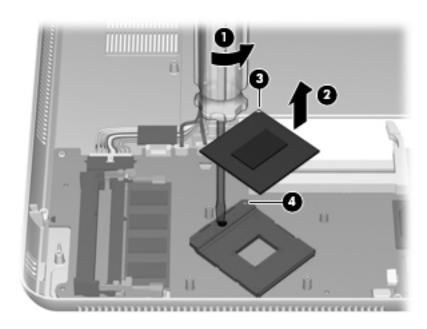
Reverse this procedure to install the processor.
