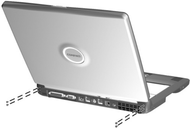
Figure C-2. Torx T8 M2.5 × 7.0 Screw Locations
