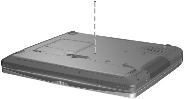
Figure C-8. Torx T8 M2.5 × 16.0 Screw Locations
