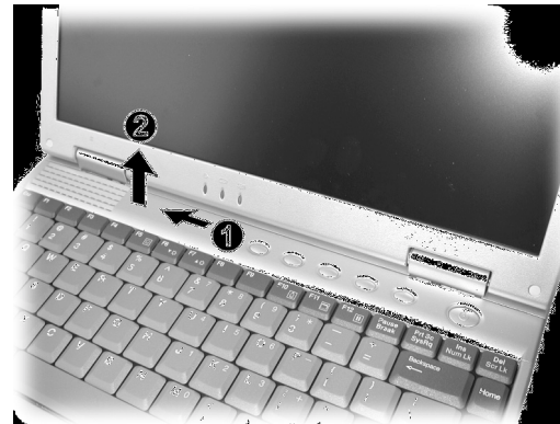
Figure 2-3 Remove LED Panel
