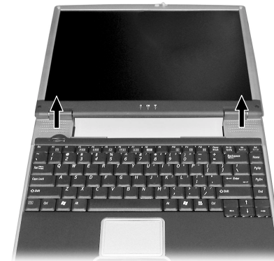
Figure 2-3 Remove the speaker cover
