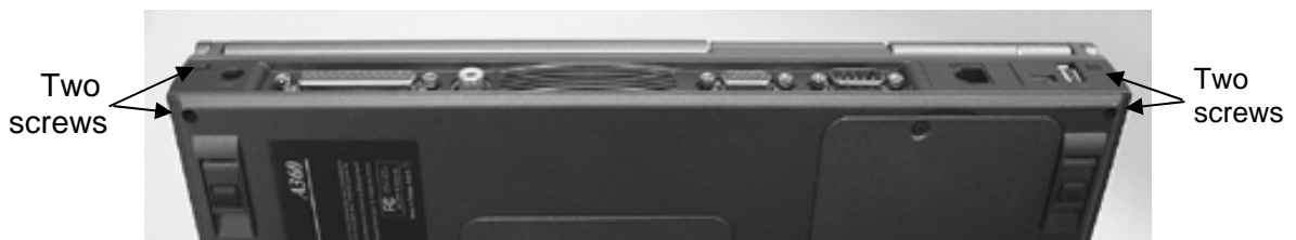
Figure 5-9 Four Screws Securing the LCD Hinges
