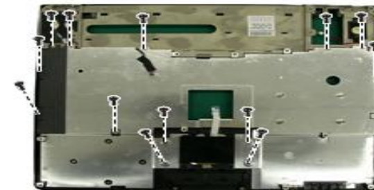
Figure 1-29 Free the touch pad
