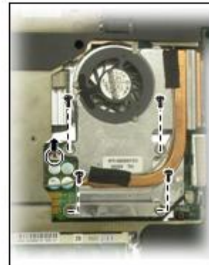
Figure 1-7 Free the heatsink
