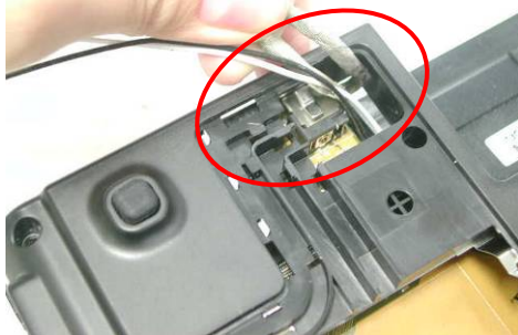
Inverter & camera cable
