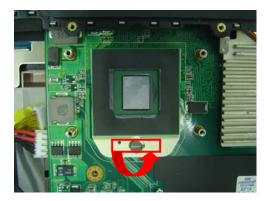
6. Remove 2 screws [M2 \*3(L)] and disconnect the fan cable & DC-in cable & Bluetooth cable, and then take the FAN module away.
