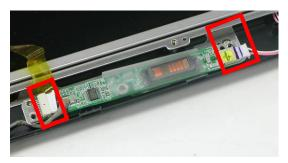
4. Remove 2 screws [M2.5 \* 8(L)] and remove the LCD bottom bracket from the LCD cover.
