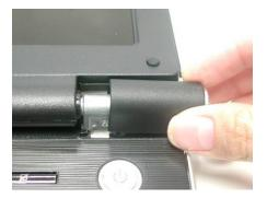
6. Remove 2 screws [M2.5 \* 8(L)] to unloosen the hinge.
