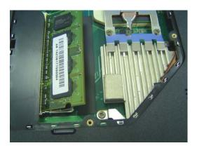
3. If there is an existing memory, remove it by opening the latches(No. 2), which will pop the module up to a 45° angle, and then pulling out the module in that angle (No. 3).
