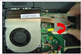
2. Turn the non-removable screw 180 degrees counter-clockwise to loosen the CPU. Squeeze the vacuum handling pump and use it to lift the CPU away.
