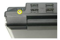
5. Remove 2 screw [M2 \* 6(L)] and carefully remove the hinge cover on the both side.
