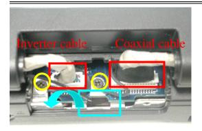
4. Remove 2 screws [M2.5 \* 8(L)] on rear side.
