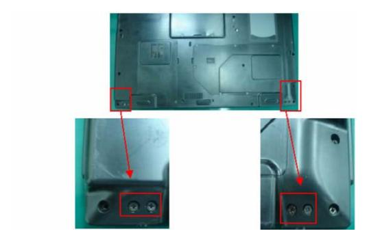
8. Separate LCD Module from the Top case module.
