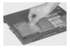
5. Reinsert the CPU board at CN17 of the system board by aligning the CPU board with the two pillars of the MMO shield as shown below.
