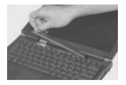
4. Lift the keyboard up and outward to expose the keyboard connector at CN20.
