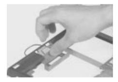
3. Remove the two screws from the left channel speaker, then lift it away.
