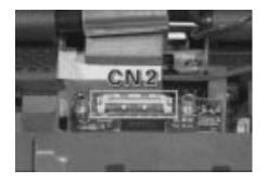
4. Remove the LCD FPC cable cover from the system board.
