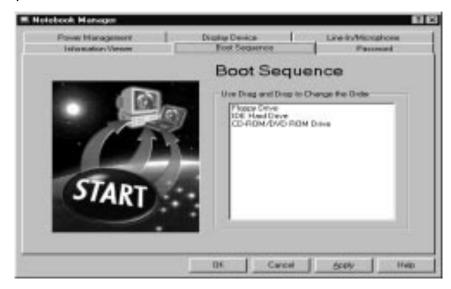
The Boot Sequence screen displays the bootable devices in your computer and the order in which the booting sequence will occur. The devices include the following:
