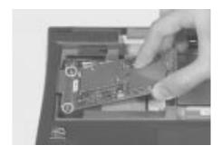
6. Use this special tool to press down and completely connect the CPU board to its socket.
