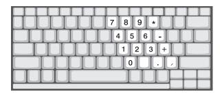
The embedded numeric keypad functions like a desktop numeric keypad. It is indicated by small characters located on the upper right corner of the keycaps. To simplify the keyboard legend, cursor-control key symbols are not printed on the keys.
