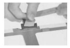
13. Disconnect the LCD FPC cable from the LCD.
