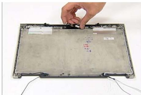
6. Grip the WebCam Module and lift upward to remove.
