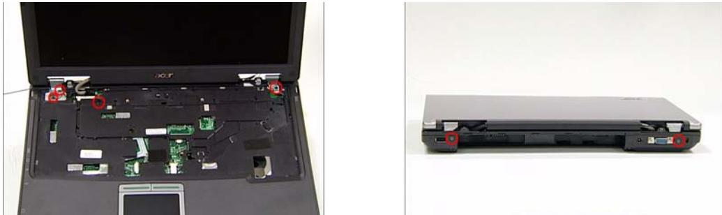
**Note:** The earth wire is disconnected when the screws are removed.
