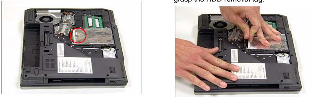
3. Pull upward as shown to remove the HDD from the chassis.
