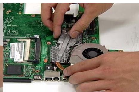
4. Align the Heatsink Securing Bracket correctly and fix in place using the two screws provided.
