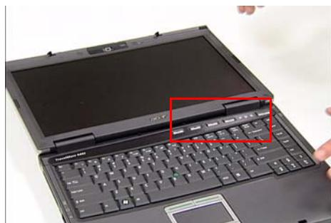
**Note:** Two of the screws are located within the battery cradle.
