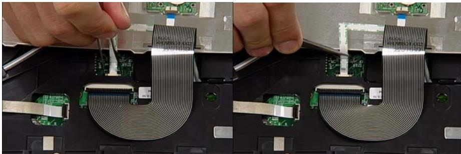
5. Using fine tweezers, release the second cable lock as shown and remove the cable from the socket.
