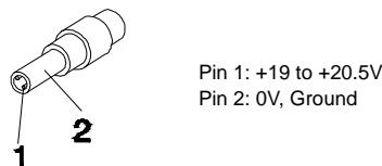
1. If the voltage is not correct, replace the power adapter.
