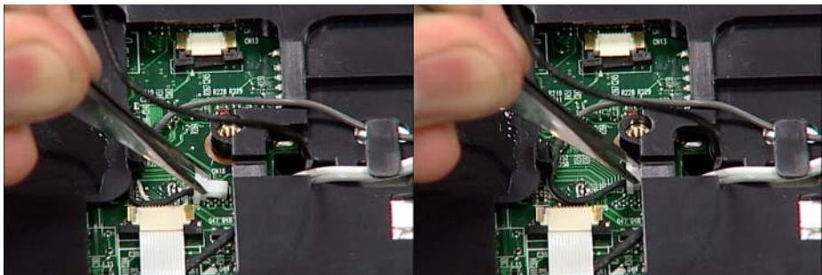
4. Turn the computer over. Place the three cables from the LCM Module in the wiring conduit and secure in place using the cable pins on the chassis.
