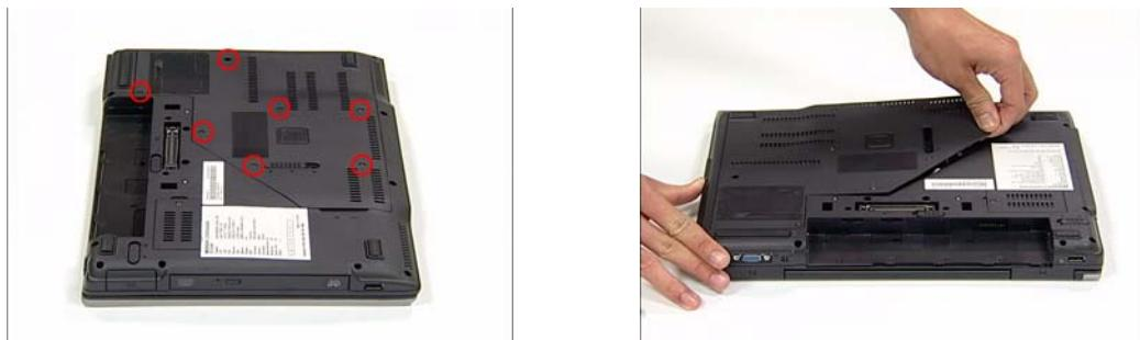
**Note:** It is not necessary to remove the screws from the CTO Cover.
