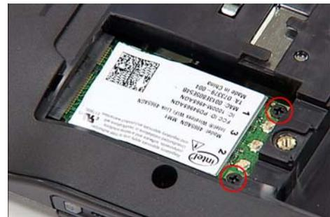
**Note:** The card remains at an angle until the screws are inserted.
