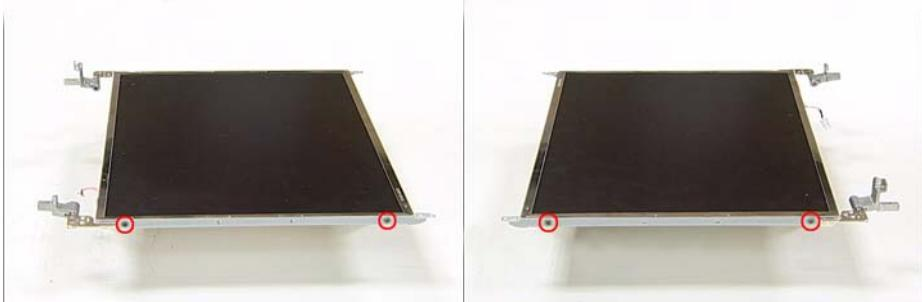
10. Remove the LCD brackets by pulling away from the LCD Panel as shown.
