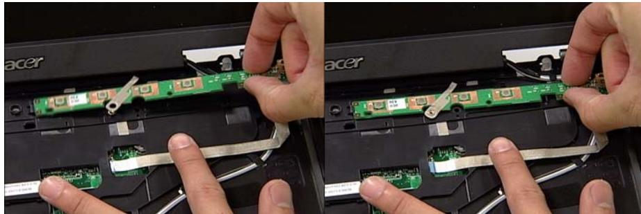
2. Insert the cable into the port and secure the locking latch using fine tweezers.
