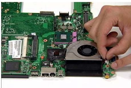
6. Remove the Fan Module by lifting straight up.
