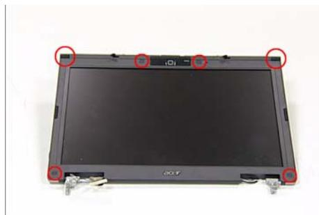
2. Loosen the bezel by lifting all the edges upward as shown.
