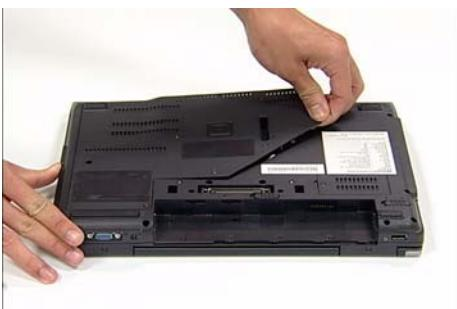
2. Push down fully until no gaps are visible between the CTO Cover and the chassis.
