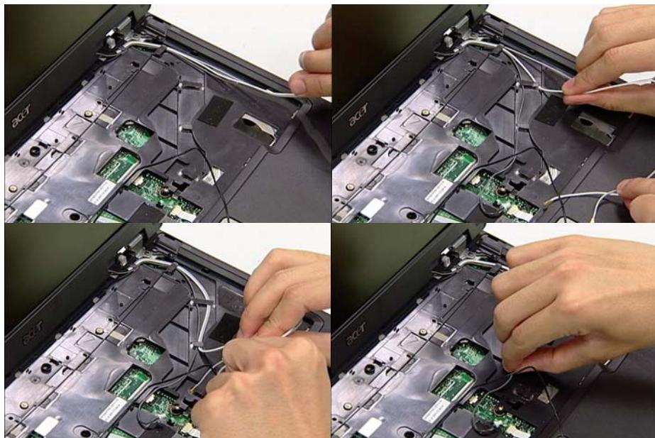
2. Push the black MIC cable from the left hand side of the computer, the white cable and the gray cable through the Mainboard so that they are accessible from underneath the computer.
