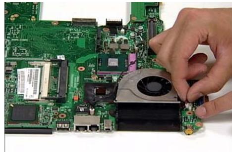
3. Hold the Fan Module in place and place the Heatsink as shown.
