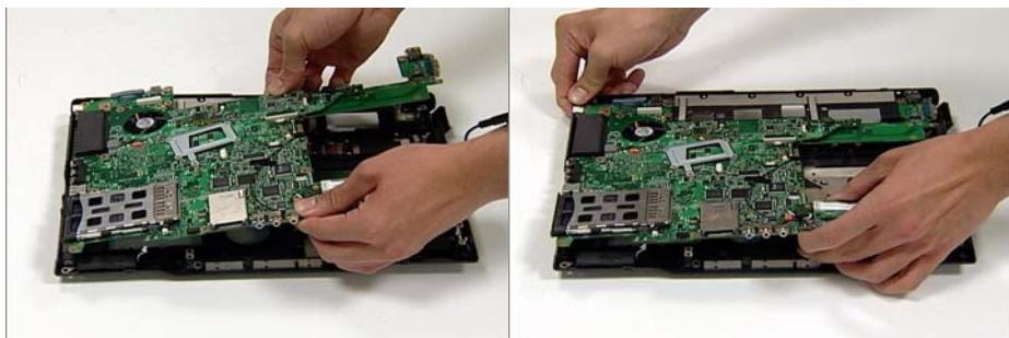
2. Close the VGA Port and connect the two speaker cables to the Mainboard as shown.
