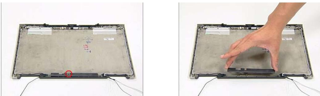
5. Grip the Inverter Board and lift upward to remove.
