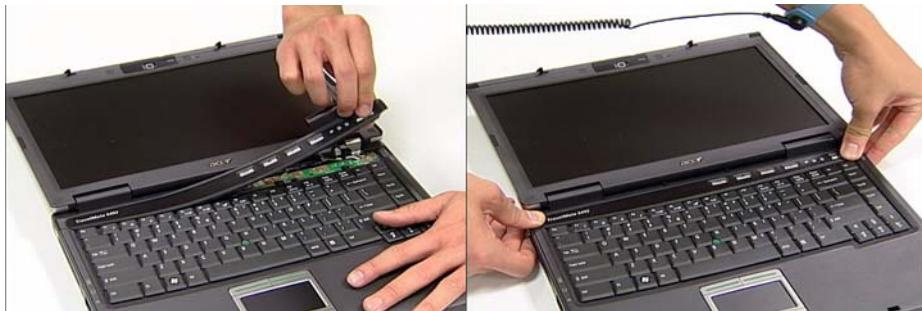
2. Close the LCM Module and turn the computer over. Locate and replace the four screws as shown.
