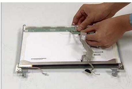
4. Align the LCD Panel cable as shown and press down to engage the adhesive pads.
