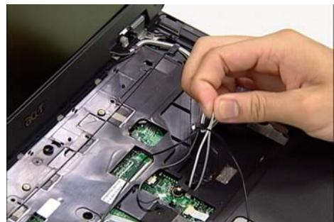
**Note:** This cable is not attached to the LCM Module. Move the cable out of the work area to avoid damage.
