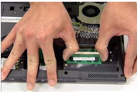
4. Pull the lower memory module away from the socket.
