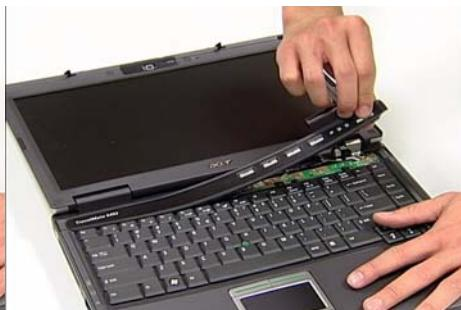
4. Using two hands, remove the Switch Cover from the chassis.
