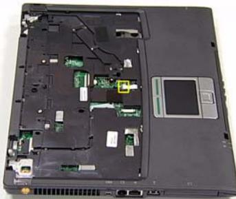
2. Using tweezers, release the locking latch and disconnect the cable as shown.
