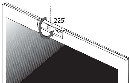
For your convenience, the camera snaps 45 degrees to match the position of your face in front or at the back of the LCD panel.
