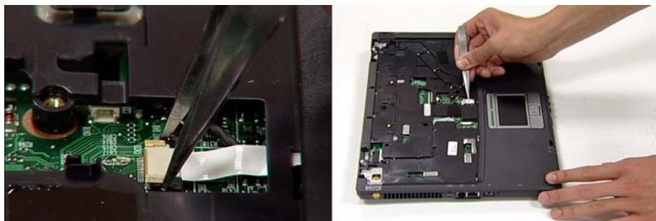
3. Using both hands, remove the casing and TouchPad as shown.
