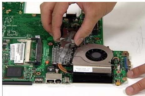
4. Hold the Fan unit with one hand and remove the Heatsink as shown.
