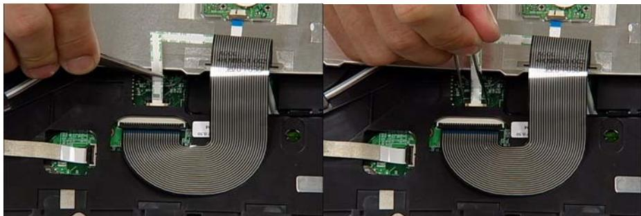
3. Turn the keyboard over and place the front edge first into the mounting.
