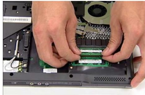
3. Push the two release levers on the lower module outward as shown.
