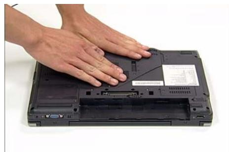
3. Secure the CTO Cover using the seven screws provided.
