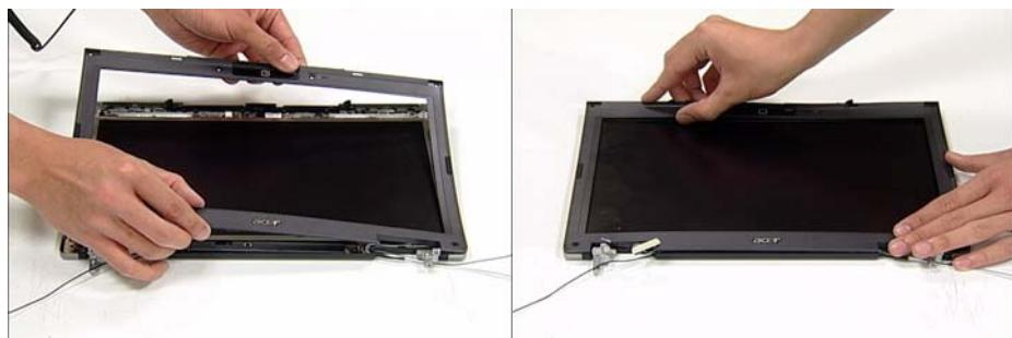
2. Secure the six screws provided and replace the mylar (small red markers) and rubber screw caps (large red markers).
