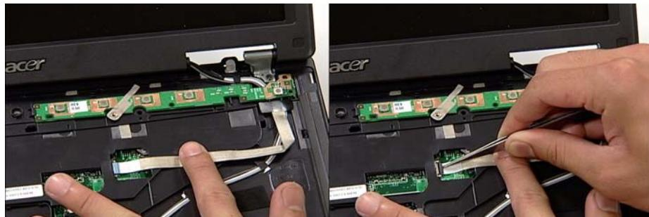
3. Secure the Switch Board in place using the screw provided.
