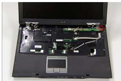
2. Using fine tweezers, release the cable lock as shown and remove the cable from the socket.
