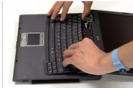
3. Turn the keyboard over, as shown, to expose the cables.
