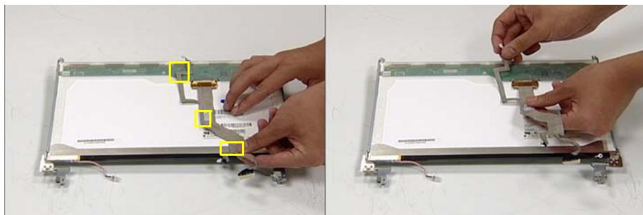
7. Turn the LCD panel over to expose the rear. Grip the LCM cable and lift upward to detach the adhesive pads.
