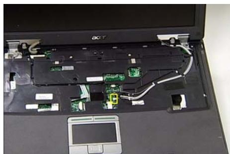
3. Using fine tweezers, disconnect the cable as shown.
