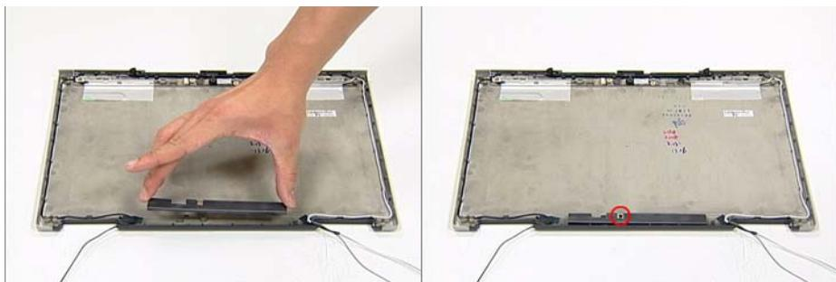
7. Place the LCD Panel in the mounting and secure the three panel connectors as shown.
