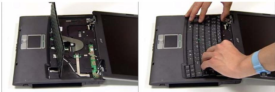
4. Push the Keyboard into place toward the TouchPad and secure using the two screws provided.
