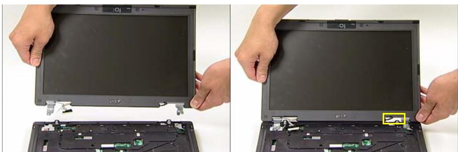
2. Connect the LCM Module cable to the connector on the chassis as shown.
