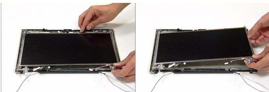
4. Locate and remove the Inverter Board screw as shown.
