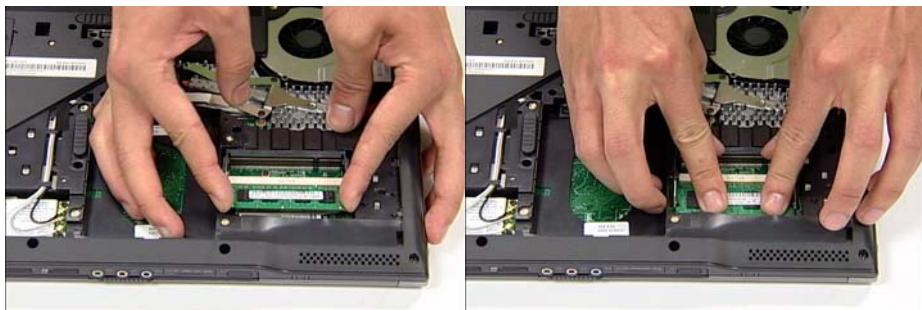
2. Using two hands, push the upper module into the socket and press downward until it clicks into place.
