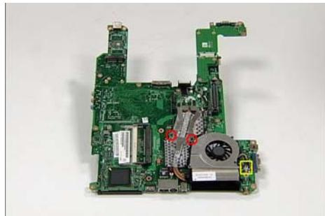
3. Remove the two screws and the Heatsink securing bracket as shown.
