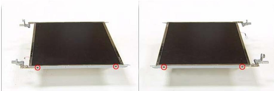
3. Turn the panel over. Insert the cable into the cable connector on the LCD Panel as shown.
