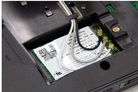
3. Locate the two screws securing the Wireless Card.
