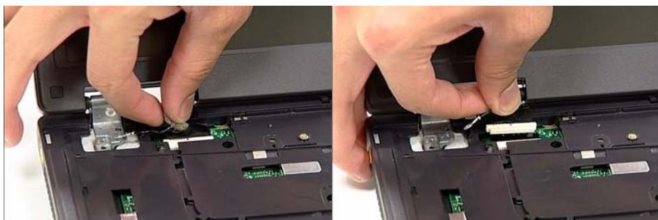
4. Using two hands, lift the LCM Module clear and remove from the chassis as shown.
