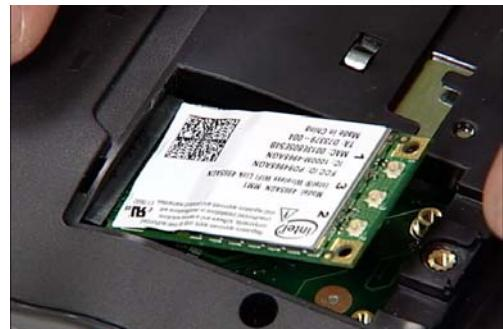
**Note:** The Wireless Card lifts up automatically once the screws are removed.
