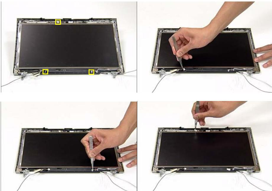
3. Hold down the WebCam Module and remove the LCD panel by lifting the hinge as shown.
