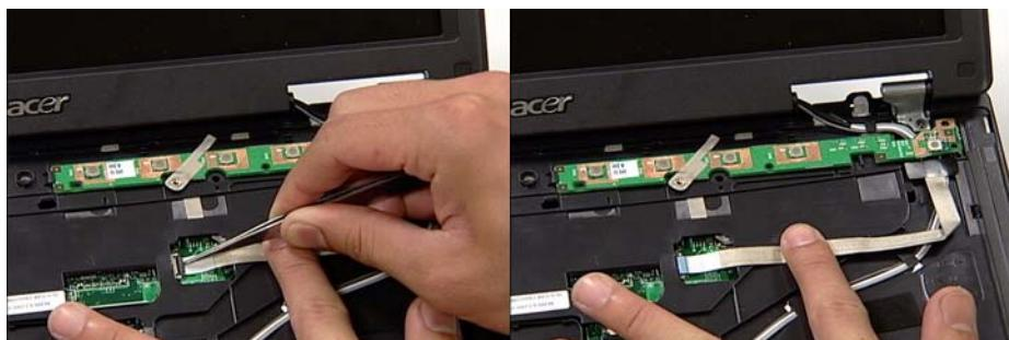
3. Remove the Switch Board from the chassis.
