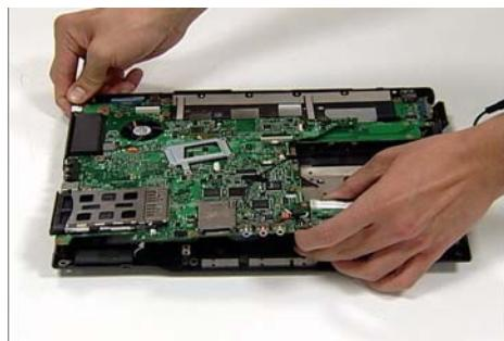
5. Lift the mainboard clear of the chassis.
