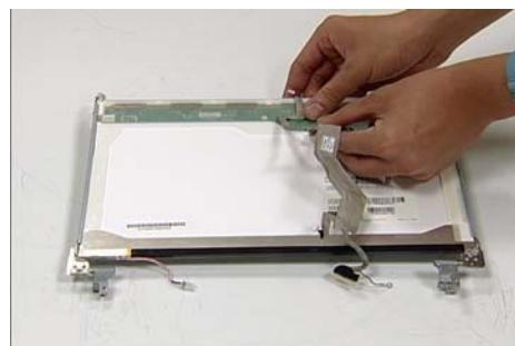
8. Hold the printed circuit board with one hand and disconnect the cable by pulling away from the connector.
