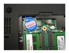
**NOTE:** RTC battery has been highlighted with the yellow circle as above image shows. Please detach the RTC battery and follow local regulations for disposal.
