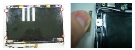
35. Remove LCM cable on the back of panel.
