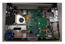
**14.** Remove the FFC of the panel and audio board.
