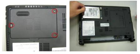
4. Remove the screw on RAM cover and remove Both of RAM
