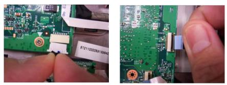
16. Remove the connector of camera and the FFC of card reader board.
