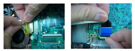
15. Remove the FFC of Bluetooth and SSD board.
