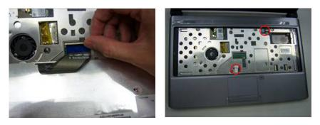
7. Remove Touch Pad FFC and lamp FFC.
